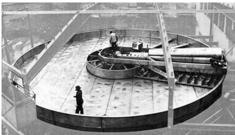
FIGURE 27.14 A 49-ft diameter DAF (Krofta Supracell) clarifier with a flow capacity of US 5650 gpm or 21.5 m 3 /min.
