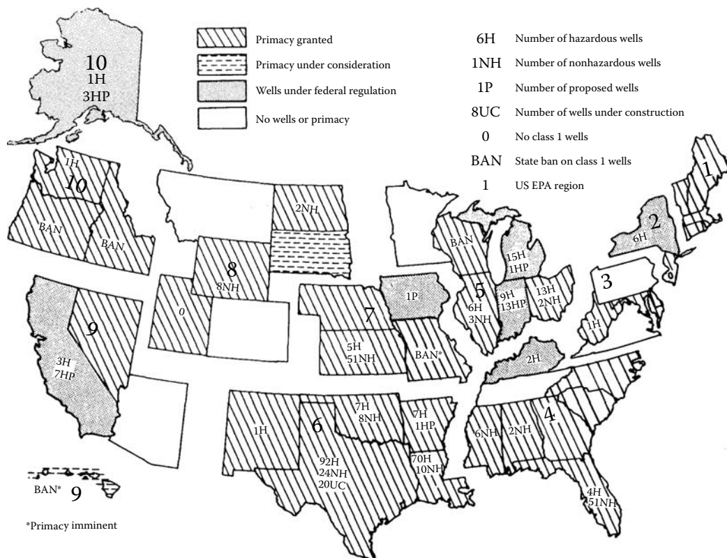
FIGURE 20.1 Regulatory status and number of Class I wells in the U.S. (From U.S. EPA, Assessing the Geochemical Fate of Deep-Well-Injected Hazardous Waste: A Reference Guide, EPA/625/6-89/025a, U.S. EPA, Cincinnati, OH, June 1990.)
